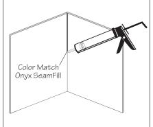
To help clean up any excess silicone, have a bottle of Rubbing Alcohol and a roll of paper towels available.
