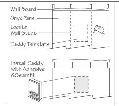
Always check for stud location before cutting the panel. If there are no studs in the intended area for the caddy, but the exact stud location is not known, begin with a small hole and then measure over to the stud for the exact location.
