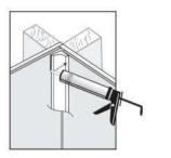
To smooth out a seamfill bead with your finger, dampen a paper towel with rubbing alcohol and then dampen your finger. Next, run your finger along the bead of seamfill, wiping any excess silicone onto the paper towel.
