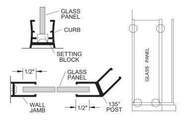
Hold the two 135° posts [**K**] plumb and carefully measure horizontally from the top of each wall jamb [**E**] to the outside edge of the posts. Add 3/16" to each measurement to find the corresponding dimension on the header assembly [**D**] (from the outside mitered edge to the squared ends) and trim the header assembly to fit.
