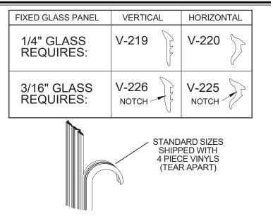
Cut eight pieces of the smaller vinyl [JJ] 1" longer than the vertical opening (to prevent gapping from shrinkage) and trim the ends on a 45° angle. Using the masking tape guides, center the first glass panel [J] in the frame. Cut four short (1" - 2") pieces of the small vinyl and press into the jamb and post on each side to hold the glass temporarily.
