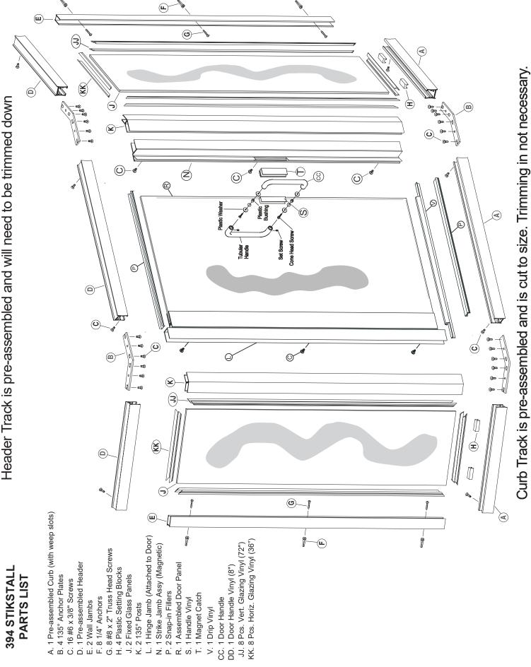
The ALUMAX 394 STICK STALL Shower Enclosure is completely reversible and may be installed pivot-left or pivot-right. For maximum waterproofing, the pivot jamb should always be opposite the shower head. Using the illustration, determine the correct position for the door in your particular STICK STALL installation. This instruction sheet depicts a pivot-right installation.
