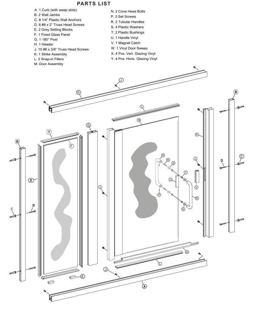
The shower door is completely reversible and can be installed hinge-left or hinge right.
