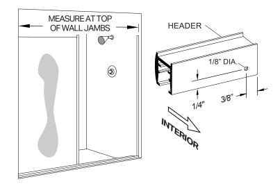
$^{\ast}\,$  Press header (H) over the wall jambs (B) and the 180°post (G).
