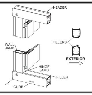
\* Remove tape and plumb door assembly laterally, then drill two 1/8" holes about 1/4" vertically from the header (H) and curb (A). Then screw into place using 2 #6 x 3/8" truss head screws.
