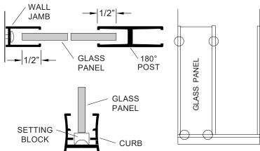
NOTE: To accommodate out of plumb walls, the 1/2" overlap may be adjusted 1/4" to 3/4"
