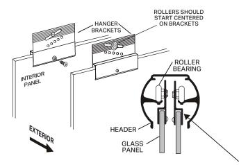
You might receive rubber pieces with the Roller Brackets to fill these gaps —These don't always fit due to tolerances, and are Never Necessary
