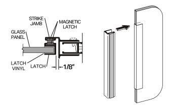
Determine the desired handing of the deflector [P]. The deflector leg must go to the inside of the unit and the notch fits under the hinge rail as shown in the drawing at right. To determine the door panel width measure the distance from the edge of the hinge rail to the far edge of the glass door panel. The deflector should be cut to Door Panel Width - 7/16". Press the deflector firmly on the bottom edge of the glass as shown.
