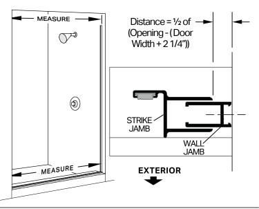
Inside the shower enclosure, drill two 1/8" holes thru the strike jamb [G] and into the wall jamb [C] 3/8" to 3/4" from the wall and approximately 1" vertically from each end of the strike jamb. Drill a third hole centered between the first two, then enlarge the three outer holes with a 3/16"drill for clearance on the self-tapping screws. Attach the strike jamb permanently with three #6 x 3/8" pan head screws [F].
