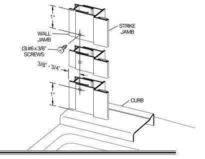
Slide the hinge jamb of the door panel assembly [B]over the mounted wall jamb [C] so the door will open outward. Adjust the door panel assembly so there is 1/4" clearance between the strike jamb and the strike edge of the glass door panel in the closed position. Mark the location of the hinge jamb on the wall jamb with a pencil.
