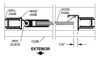
Inside the shower enclosure, drill two 1/8" holes thru the hinge jamb and into the wall jamb [C] 3/8" to 3/4" from the wall and approximately 1" vertically from each end of the hinge jamb. Drill a third hole centered between the first two, then enlarge the three outer holes with a 3/16" drill for clearance on the self tapping screws. Attach the door panel assembly permanently with three #6 x 3/8" pan head screws [F].
