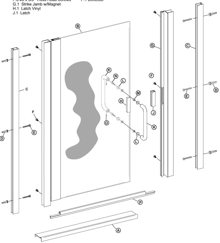
Refer to the illustration to determine the correct position for your installation. For maximum waterproofing, the hinge jamb should always be opposite the shower head. These instructions depict a hinge-left and hinge-right installation based on shower head location.
